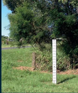
Manual staff gauge Granville Boat Ramp
