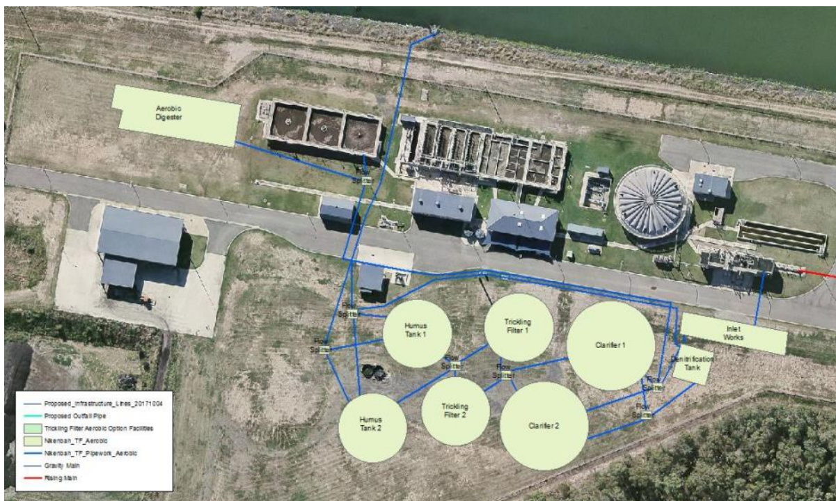
Figure 4.3 Nikenbah Trickling Filter Site Layout
