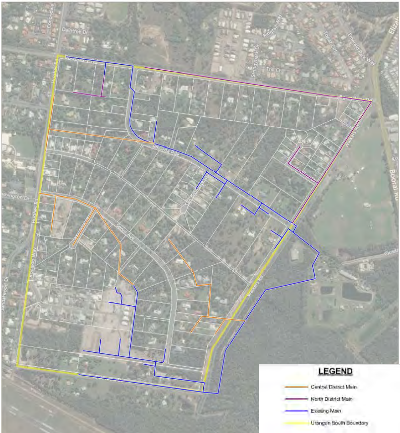
Figure 5-18 Maximum yield (existing zoning) scenario Sewer Augmentation
