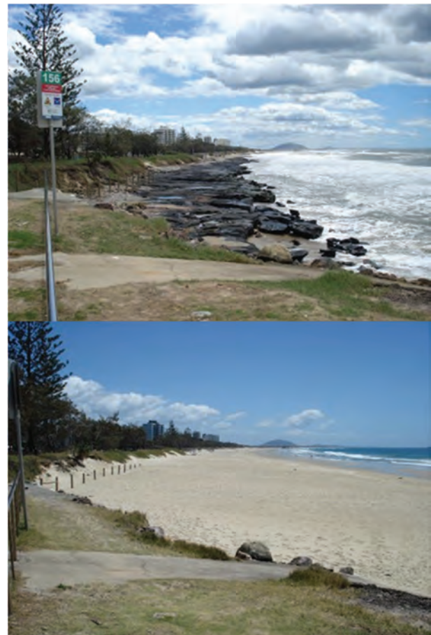
Figure 2 Maroochydoore Beach before (top) and after (bottom) a 125,000 m 3 beach nourishment campaign, September 2013 (photos courtesy of Birdon Pty Ltd)
