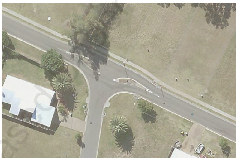
New Section - Typical Traffic Calming at entrance to cul-de-sac
