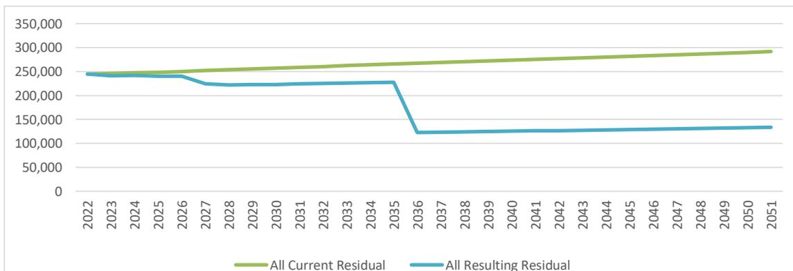
Figure 18 Impact on residual waste volumes if EfW is utilised
