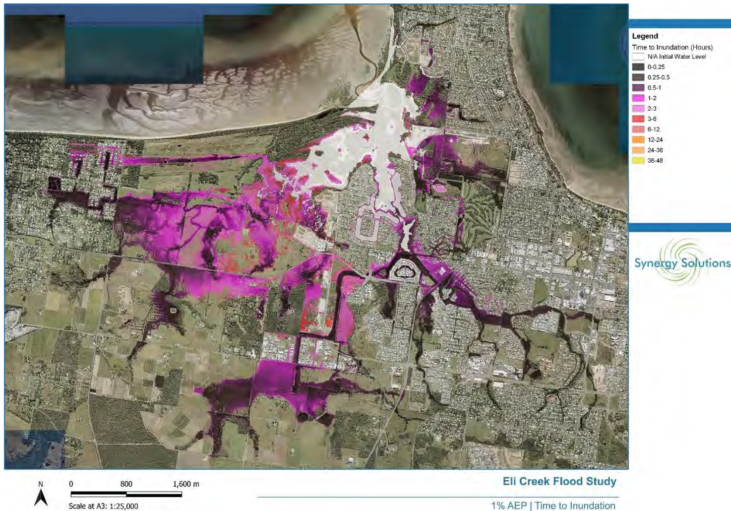
Figure 12-6 1% AEP Time to Inundation
