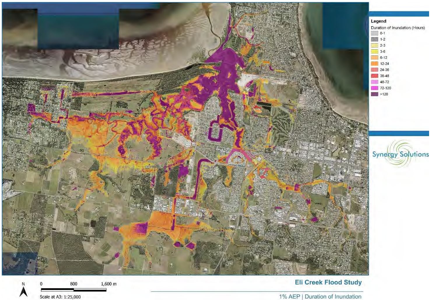
Figure 12-7 1% AEP Duration of Inundation
