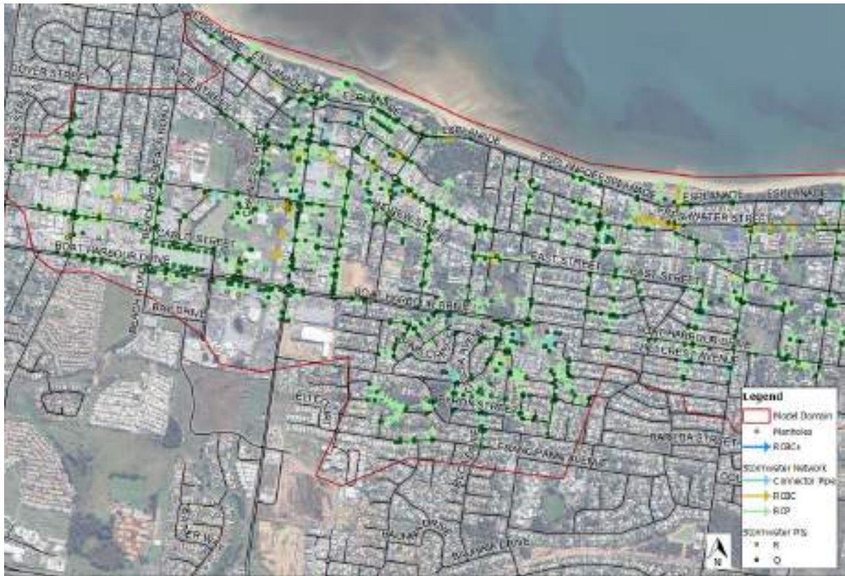
Figure 2-4 Toon Toon Stormwater Network
